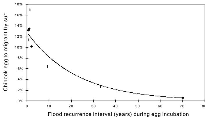
Figure 6. Chinook egg to migrant fry survival versus flood recurrence interval (years) during egg incubation in the Skagit River, Washington from 1989 to 1996 (from Pess et al. 2000). Regression equation is chinook egg to fry survival =  $0.1284e^{-0.0446(\text{flood recurrence interval})}$  ( $r^2 = 0.97$ ,  $P = 0.007$ ).
