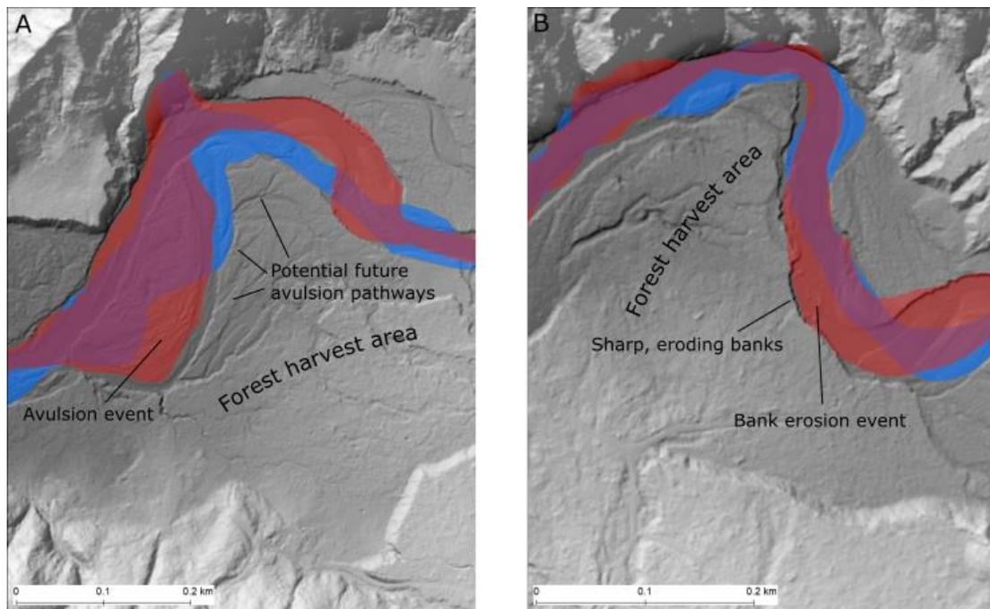
Figure 3. Example of A) avulsion and B) bank erosion hazards as seen on hillshade images of a lidar DEM. The avulsion zone in A is composed of multiple channel threads that cross the geologically-modern floodplain. In B, bank erosion is apparent in sharp banks. In both images the active channel envelope is mapped in 1998 (blue) and in 2017 (red).
