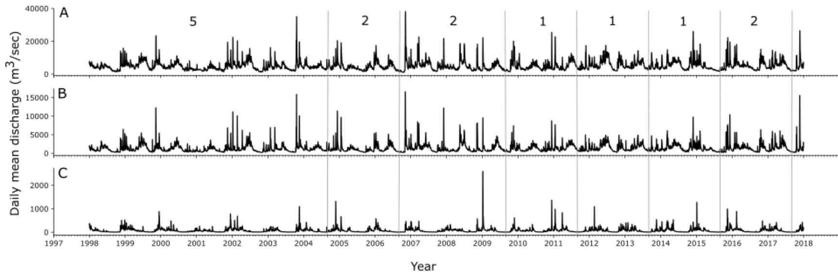
Figure 9. Mean daily discharge at three USGS gages in the Skagit and Samish River basins. A) Skagit River at Mount Vernon (lower Skagit basin); B) Sauk River at Sauk; and E) Samish River. Vertical grey lines represent the approximate date of each aerial photograph used in the analysis; the count of each FPA that experienced migration in each time period is shown at the top of the figure.
