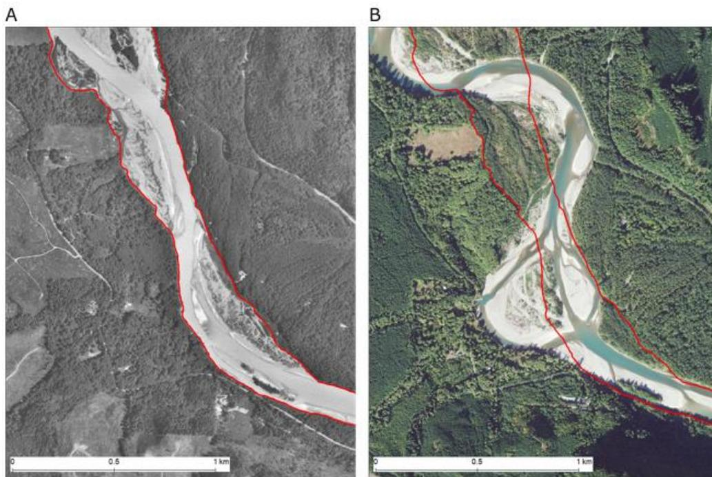
Figure 1. Aerial photographs showing channel migration in the Sauk River between A) 1998 and B) 2017. The location and scale are identical in both photos. The 1998 active channel envelope (see text) is mapped in red.
