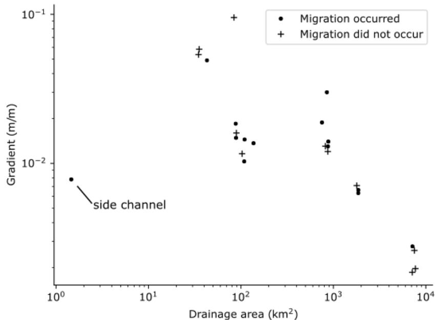
Figure 10. Channel gradient versus contributing drainage area for all study sites, stratified by migration status. The point marked 'side channel' was a side channel to the Sauk River; it had a very low slope but was effectively cut off from upstream drainage area due to the mechanics of our flow accumulation algorithm (appendix B).
