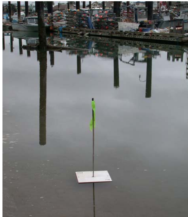
Figure D.VI.1. The drift buoy. The base is 13 inches by 13 inches, and made of plywood. The pole is a bamboo garden stake. The base has a four-ounce fishing weight attached for displacement.
